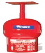
PD-Matic is a newly developed product, where in the Dry Powder is automatically ejected through the sprinkler head, after release of the thermo safety device on reaching a temperature of 68°C.
